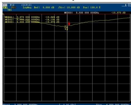
Gambar 16 Hasil Pengukuran ReturnLoss Input
