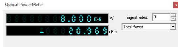
Gambar 7 Daya Terima Receiver Downstream
