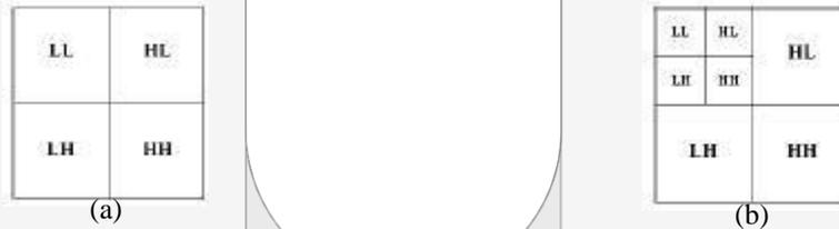
**Gambar 1 (a) DWT Level 1 [3] (b) DWT Level 2 [3]**
