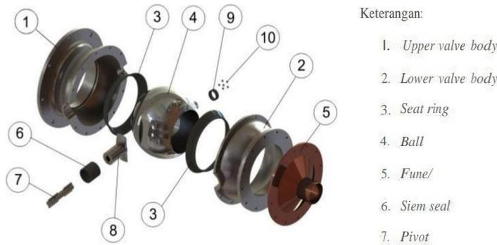
Gambar 3 *Komponen valve tea bulker*
