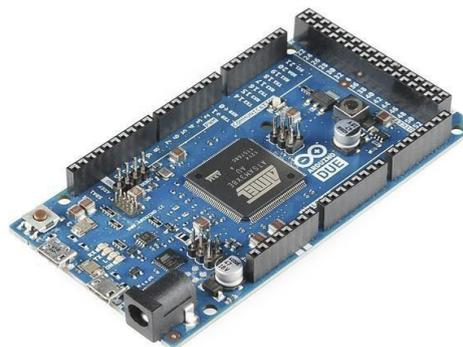
Gambar 5. Arduino Due
