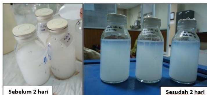
Gambar 3.4 Sedimentasi nanofluida Air- \text{Al}_2\text{O}_3 .
