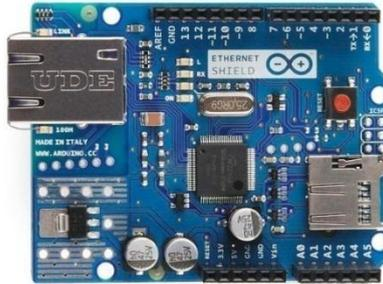
Gambar 3 Ethernet Shield
