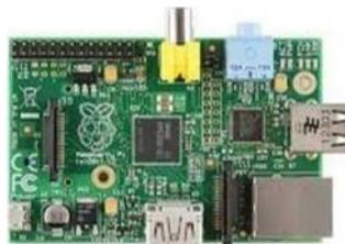
Gambar 2 *Error! No text of specified style in document.* 1 Raspberry Pi ver B
