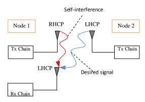
Fig. 1. Proposed Self-Interference Cancellation Model
