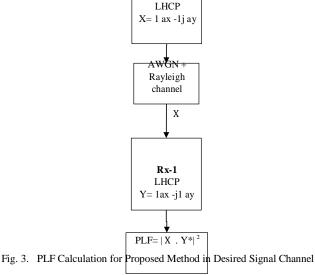
Based on Fig. 3, the channel is not FSL, so the PLF value is in range between 0 and 1, but the PLF value in this model is higher than the PLF value in Fig.3 if the channel is AWGN, it because of using the different polarization
