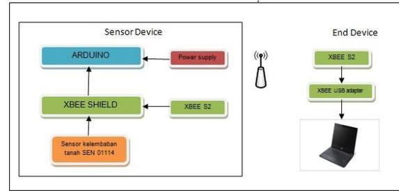
Gambar 3. 1 sensor device
