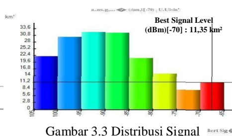
Gambar 3.3 Distribusi Signal Coverage Bandung - Cikampek
