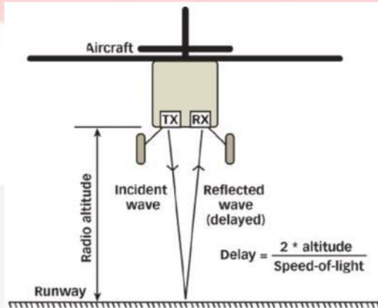
Gambar 1 Ilustrasi Radio Altimeter<sup>[8]</sup>
