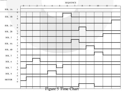
Time chart shows the devices or actuator active on each sequence. It will help to troubleshooting or configuring the devices by seen the chart. Time chart also represent the sequence of device work based on PLC program then it can easier to check what device is not working properly.
