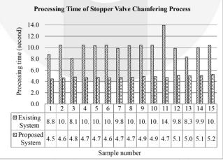
Figure 6 Processing Time of Stopper Valve Chamfering Process
