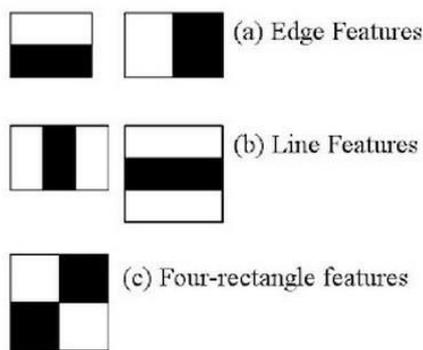
Gambar 2.2 Haar-like feature (Source : [http://docs.opencv.org/trunk/doc/py\\_tutorials/py\\_objdetect/py\\_face\\_detection/py\\_face\\_detection.html](http://docs.opencv.org/trunk/doc/py_tutorials/py_objdetect/py_face_detection/py_face_detection.html))
