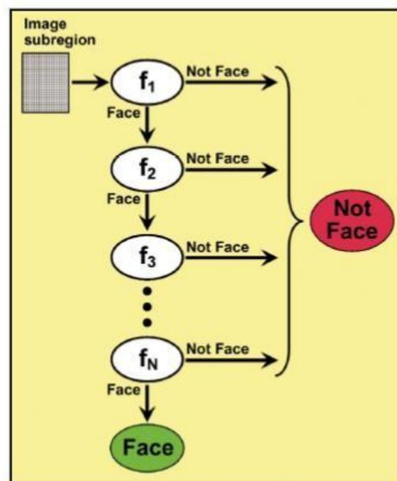
Gambar 2.4 Proses cascade classifier (Source : [http://www.cognotics.com/opencv/servo\\_2007\\_series/part\\_2/sidebar.html](http://www.cognotics.com/opencv/servo_2007_series/part_2/sidebar.html))
