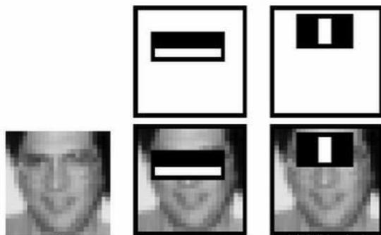
Gambar 2.5 Contoh pencarian dengan haar-like feature (Source : [http://docs.opencv.org/trunk/doc/py\\_tutorials/py\\_objdetect/py\\_face\\_detection/py\\_face\\_detection.html](http://docs.opencv.org/trunk/doc/py_tutorials/py_objdetect/py_face_detection/py_face_detection.html))
