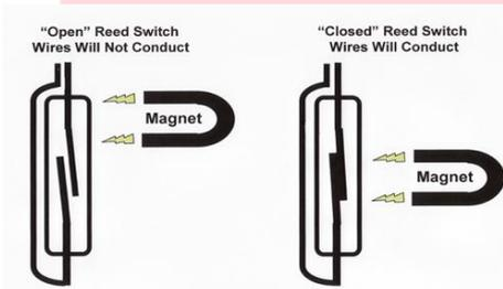
Gambar 2.7 Reed switch and magnet<sup>[6]</sup>
