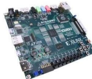
Gambar 4.18 Spartan-6 XC6SLX45 CSG324C<sup>[10]</sup>
