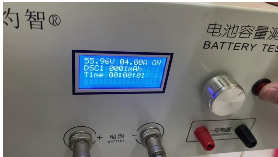
Figure 4. 4 Regenerative Braking System Load Testing Using a Battery Tester
