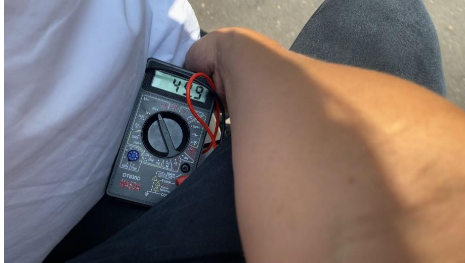
Figure 4. 2 Voltage Output Check of the Regenerative Braking System
