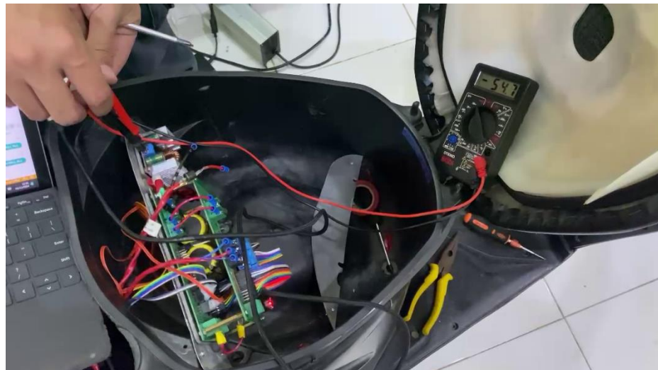
Figure 4. 3 Voltage Check of the System with Step-up
