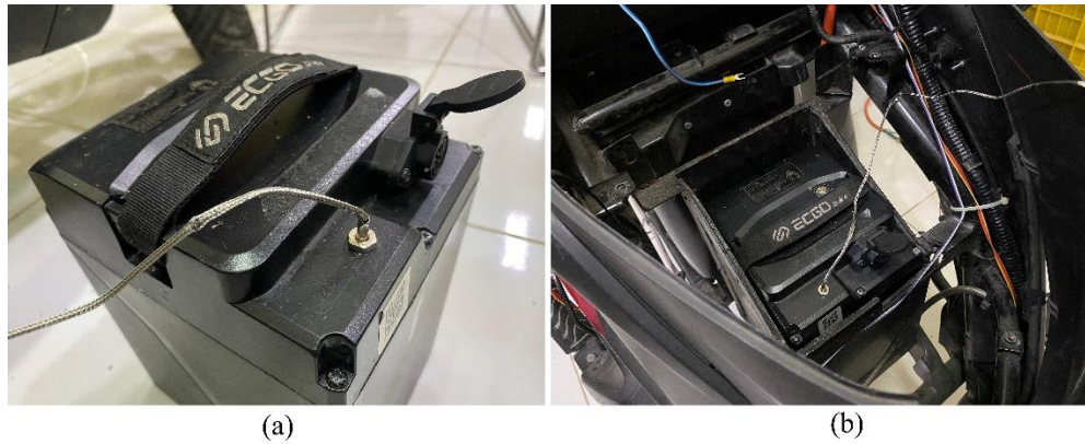
Figure 3. 6 (a) Temperature Sensor Position, (b) Battery Position
