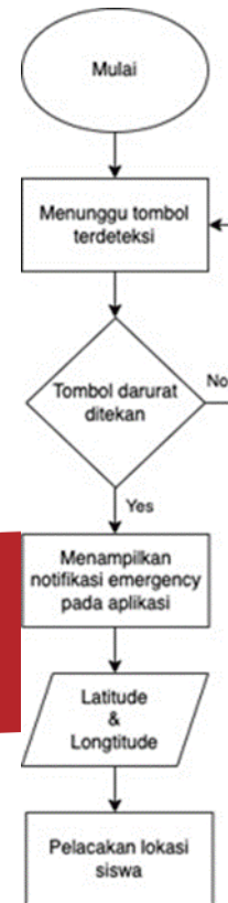
Gambar 4 Flowchart Emergency Button
