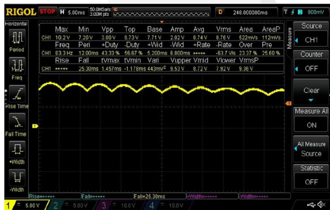
Gambar 4.3 Hasil pengujian Three Phase Rectifier tanpa kapasitor
