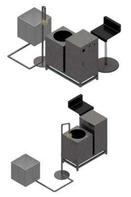
The final machine has an additional part that come from Concept D, with the change of the chair. The place where it places the water on the jug is now being automatically given from the pipe to the brush which also automatically turn for cleaning on the jug inside.
