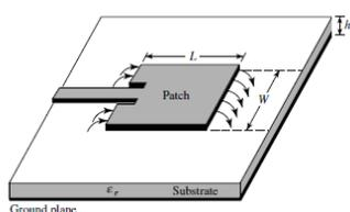
Gambar 1. pencatutan *Microstrip line feed*<sup>[8]</sup>
