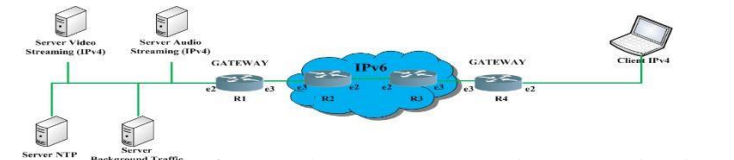
Gambar 3.5 Topologi Skenario 5 464 Tunneling Layanan Mixed Traffic Video dan Audio Streaming
