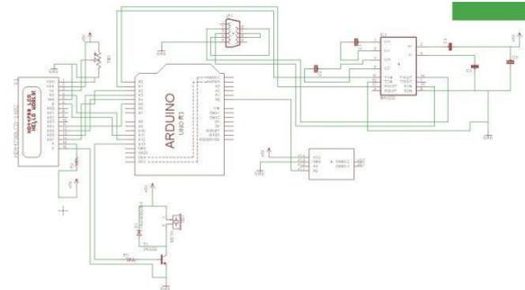
**Gambar 3.3** Schematic Rangkaian.
