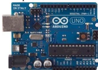
Gambar 2(a) Papan Arduino Board
