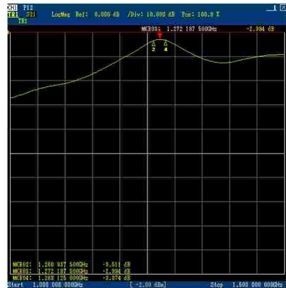
Gambar 3.2 Hasil Pengukuran Insertion Loss
