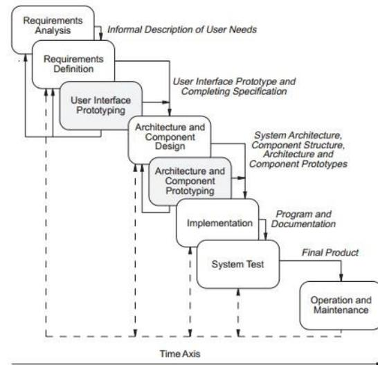
Gambar 3 Alur proses metode Prototyping
